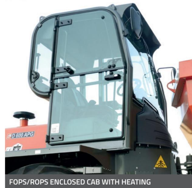
FOPS/ROPS ENCLOSED CAB WITH HEATING
